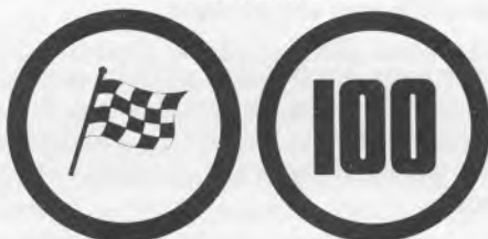
Both signs to be placed at 100 yds or 100 metres before the flying finish
